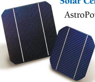
AstroPower's AP-105 and AP-106 solar cells are high-efficiency five and six inch single crystal solar cells, respectively. They are the largest and most powerful solar cells available today, rated between 1.5 and 3.3 watts each. Our new APex™ six inch polycrystalline silicon solar cells use our patented Silicon-Film™ technology for high-speed, large-area fabrication of solar cells at low cost. Large solar cells are more cost effective.
