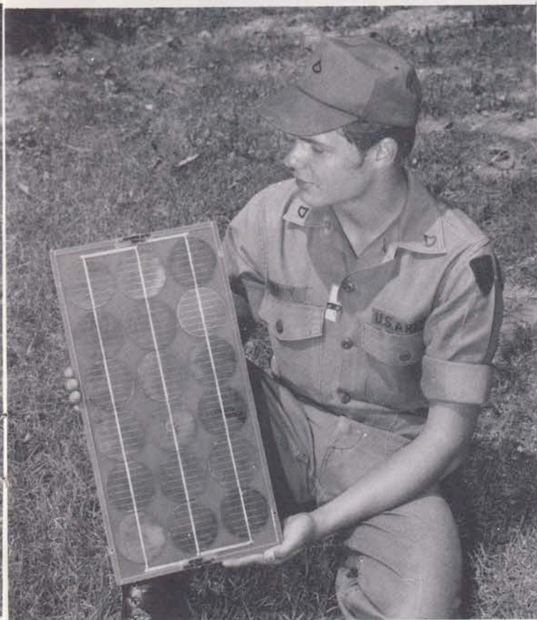
(Above) Basic 10W (peak) output solar panel comprised of 3" diameter Chevron™ silicon solar cells. This Solarex panel is a basic building block for large arrays. (Right) 460W (peak) solar electric system powering microwave and VHF repeaters in the Mojave Desert.
